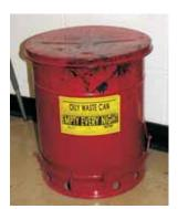
All rags that contain solvent residue should be kept in metal cans with properly fitting lids to avoid exposure to solvent vapor. Exercise extreme care when exposed to dangerous materials. Proper personal
