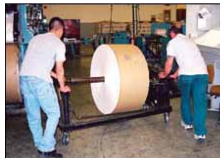
Figure 13. Using a roll cart with power lift to move rolls to press units.
